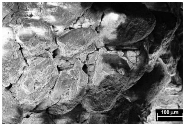
Figure 3. SEM image of the porous ceramic showing silica sand particles in the order 200 \times 10^{-6} m and larger pores between them.
